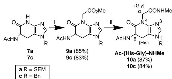
**Scheme 4.** Reagents and conditions: (i) a. NaH, THF, room temperature, 1 h. b. BrCH<sub>2</sub>CO<sub>2</sub>Me, reflux, 5 h; (ii) MeNH<sub>2</sub> (2 M in MeOH), MeOH, 16 h.
