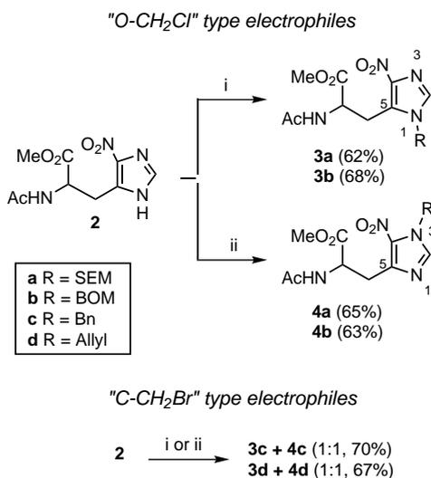
**Scheme 2.** Reagents and conditions: (i) a. NaH, DMF, 0°C, 1.5 h; b. RX, 0°C, 1 h; (ii) NaH, DMF, room temperature, 1.5 h, RX, room temperature, 1 h.
